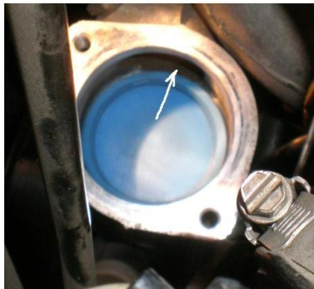
Thermostat housing with disc covering the bottom (bypass) hole
